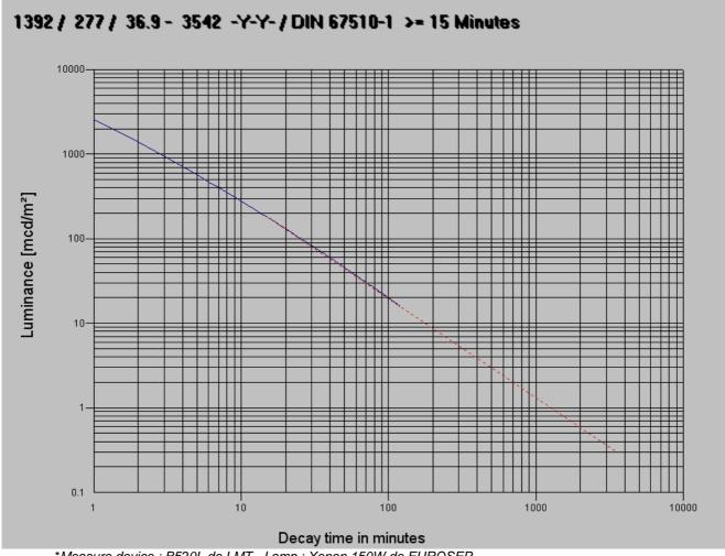
\*Measure device: B520L de LMT - Lamp: Xenon 150W de EUROSEP
